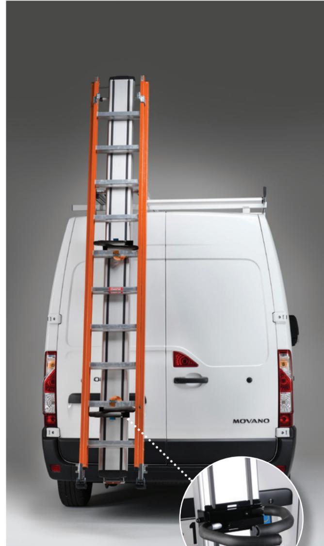
*New, improved and adjustable ladder retainers to hold the ladder firmly in position.*
