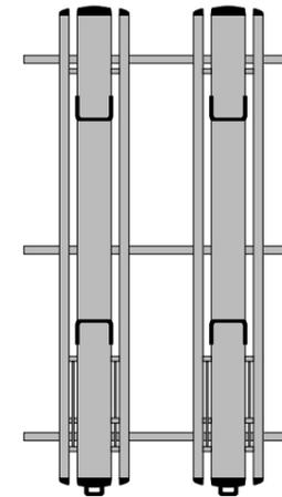
Single G2000 Harrier with Gentili roof mounting bars, side rail kit, rear roller and front spoiler
